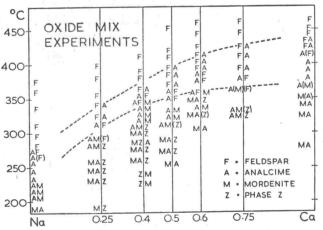
Fig. 11. Phases formed by hydrothermal crystallization of oxide mixes of feldspar compositions. (For pressure data see Appendix I).
